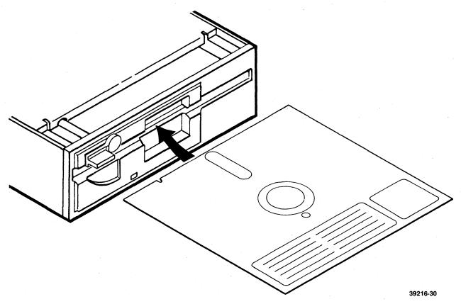
FIGURE 8-1. LOADING THE SA810/860
