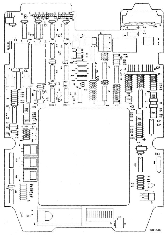
FIGURE 7-1. PCB COMPONENT LOCATIONS (P/N 25227 AND 25247)
