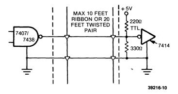
FIGURE 2-2. INTERFACE SIGNAL DRIVER/RECEIVER
