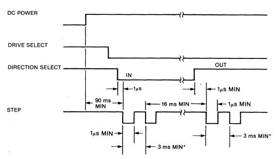
\*3 ms is the minimum frequency for a standard seek. Pulses received at less than a 3 ms frequency will go into a buffered seek mode. See figure 1-4.
