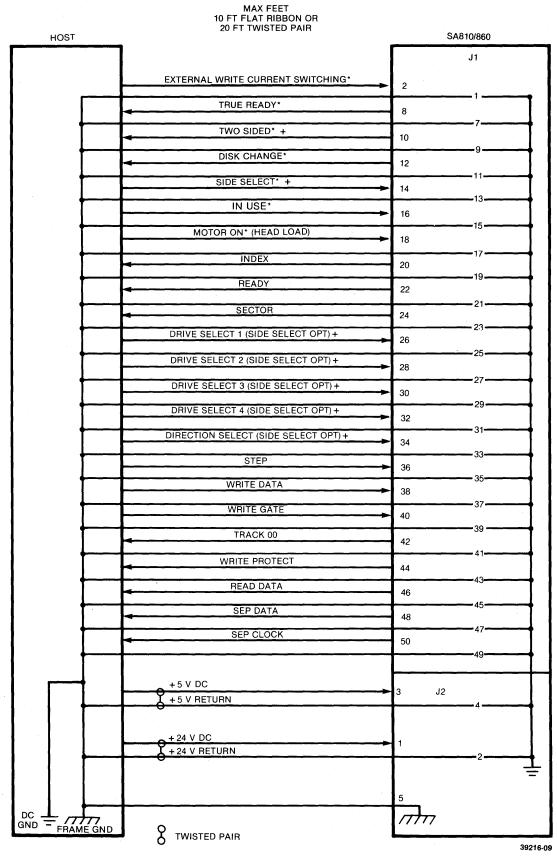
\*JUMPER ENABLED ALTERNATE I/O LINES. + SA860 ONLY
