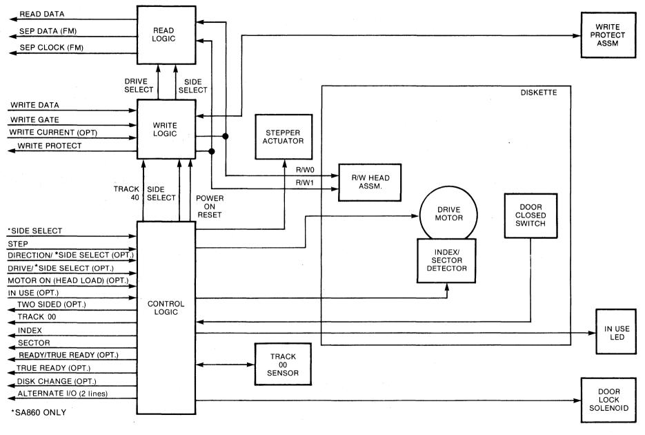
FIGURE 1-2. SA810/860 FUNCTIONAL DIAGRAM
